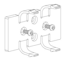
The mounting clip can be fastened to flat surfaces using Velcro, double-sided tape or screws.
