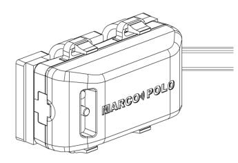
Once the mounting clip is attached to an object, the tag can be clipped into place. Be certain to align all 4 hooks in the clip with the 4 eyelets and then press firmly to fully engage the hooks.
