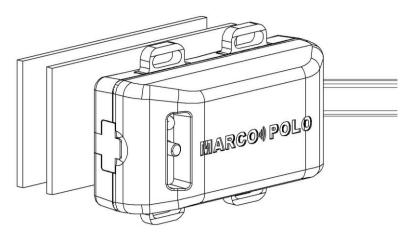
The tag transceiver can be mounted directly using zipties placed through the eyelets or by attaching to a flat surface using Velcro or double-sided tape.
