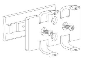
For attaching the mounting clip to curved surfaces, the supplied strut adapter can used in either the vertical or horizontal positions as shown above.
