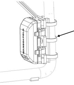
When using the strut adapter, feed zip-ties through the slots in-between the mounting clip and the strut adapter.
